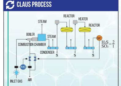
Catalysts are applied at Claus sulfur recovery units for hydrogen sulfide removal from natural and industrial gases of different origin. Catalysts ensure high activity in main Claus reaction
